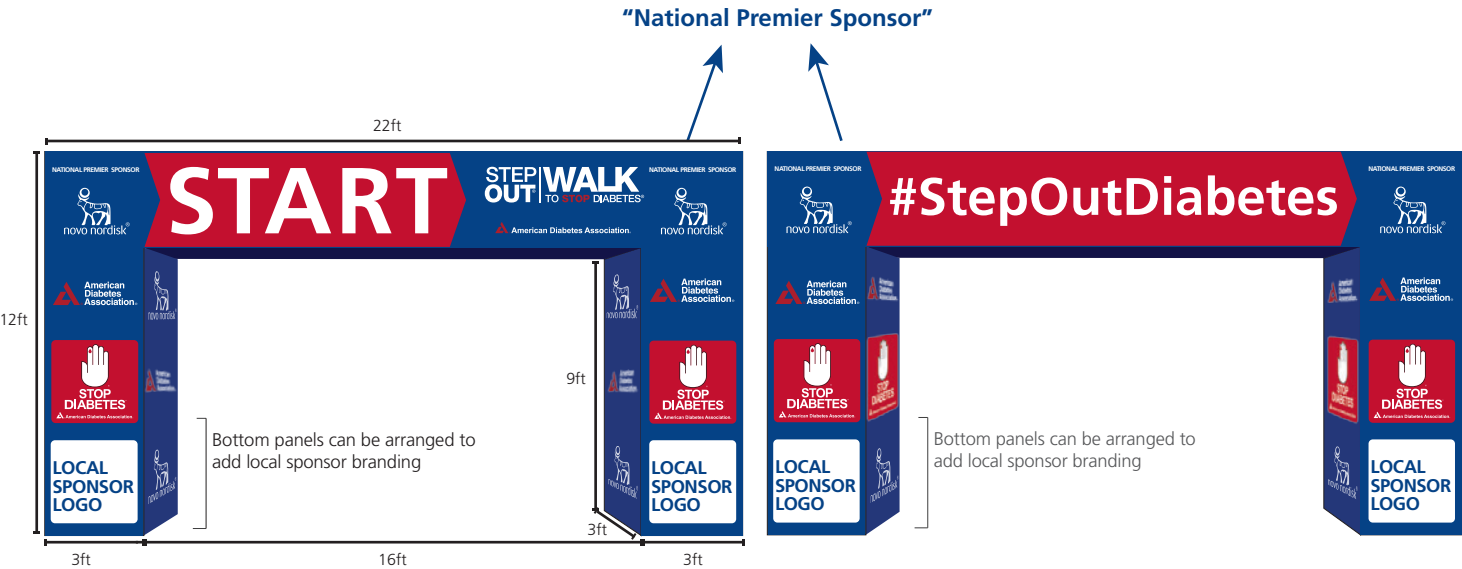
Inflatable Arch Arch Interior: 9' Tall, 16' Wide, 3' Deep Arch Exterior: 12' Tall, 22' Wide, 3' Deep
